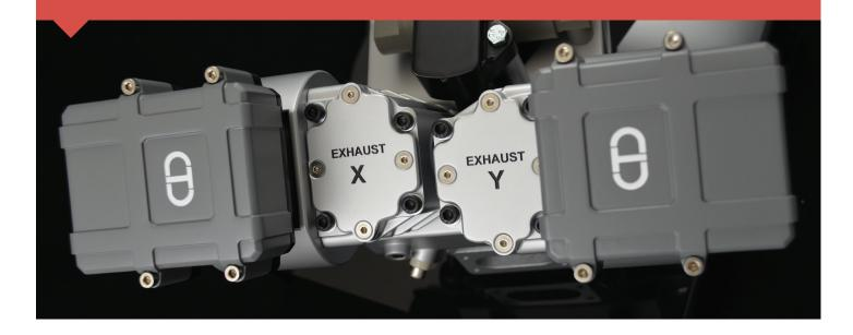
The main cylinder head was produced using SLS which not only allows for complex geometry but is self-supporting with high tensile strength. The accuracy achieved at Ogle is +/-0.12mm per 100mm.
