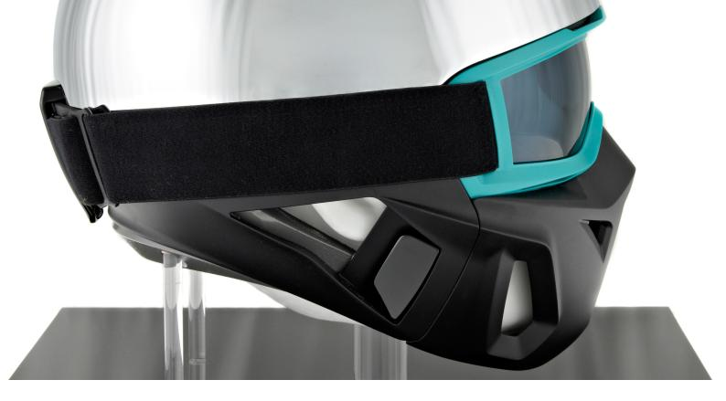
The helmet required a series of parts to be made, including goggles, lower maverick, lower shell and left and right mask clip. Ogle completed the project using Selective Laser Sintering (SLS) for the hard parts and Stereolithography (SLA) then Vacuum Casting, using silicon tools, for the clips and softer parts.
